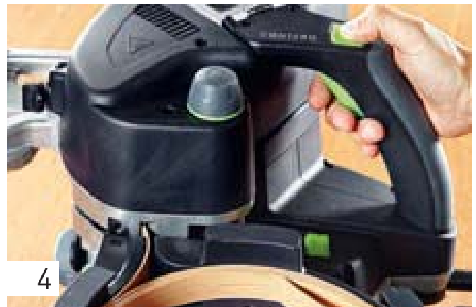
4 Start drawing the edging into the machine by pressing the start button once. Thread the edging through the gap in the edging holder and into the infeed. Gluing can begin as soon as the machine draws in the edging.
