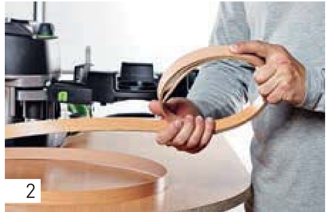
2 You must cut the edging to length first and roll it up with the visible side facing inwards because you cannot work directly from the roll in the edging holder.
