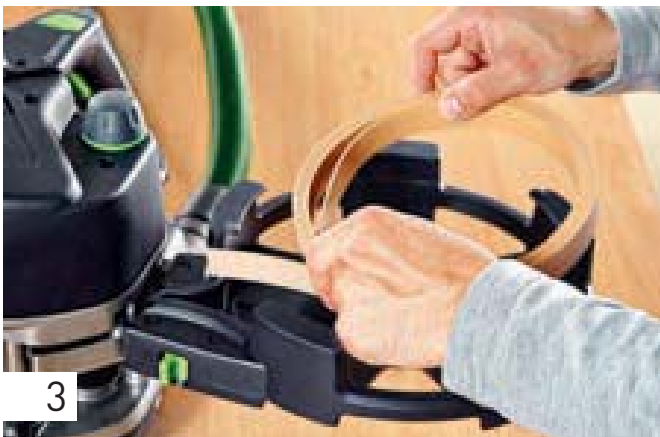
3 Place the roll of edging in the holder, positioning the end of the edging in the direction of the edging infeed on the machine.
