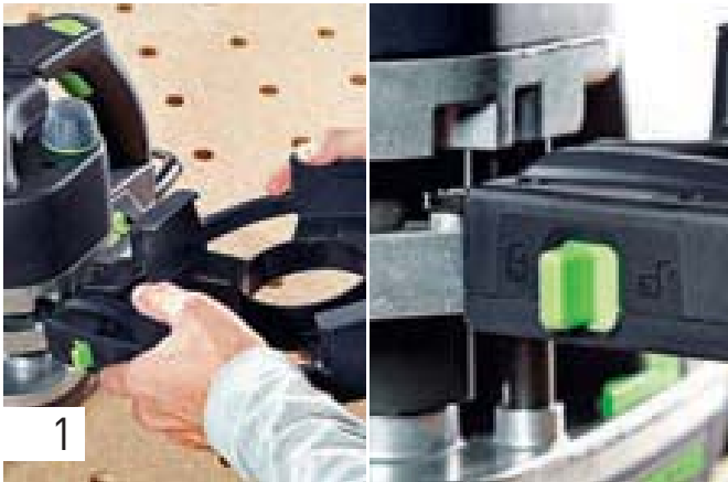
1 Mount the edging holder first of all. Simply attach to the pins provided and secure with the locking mechanism.
