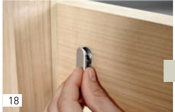
18 Optionally, you can cover the routing with a cover cap, available in one of three colours depending on the material: silver, light brown or dark brown.
