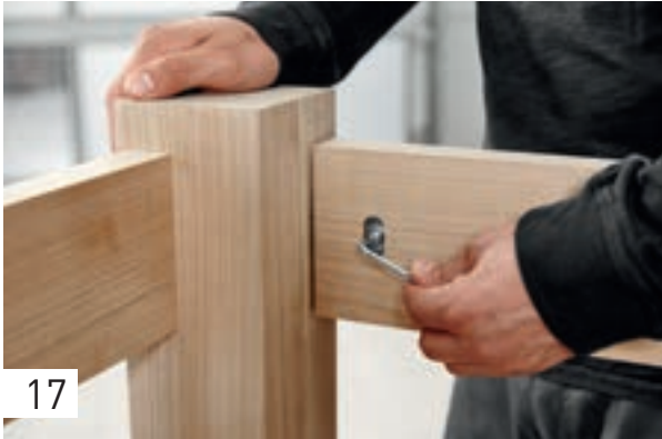
17 Tighten the connection using a 4 mm hexagonal socket.
