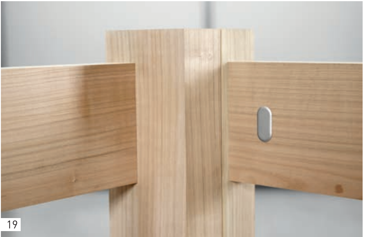
19 This is a quick way to create a stable joint that can be quickly disassembled if necessary, without time-consuming measuring or marking.
